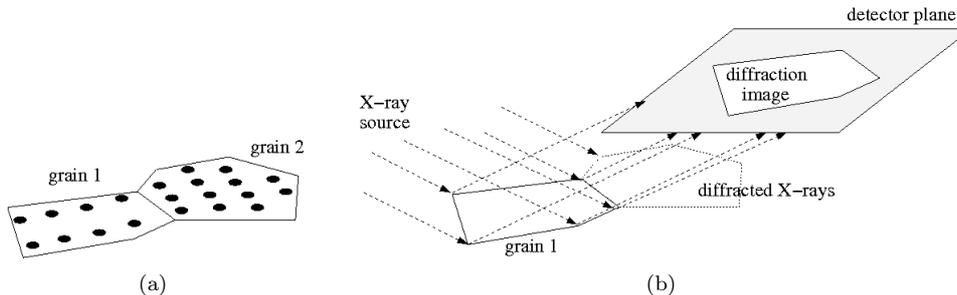
Figure 1: Schematic illustration of grains and diffraction. (a) A sample layer containing 2 grains with different lattice structures. The shapes are indicated by the polygons, the lattices by the dots – real grains contain considerably more unit cells. (b) Diffraction from a layer, assuming that only grain 1 is in diffraction condition. An affine image of its shape is recorded on the detector. The detector plane need not be parallel to the sample plane.
