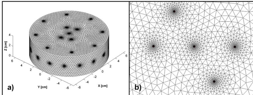
Figure 1: FEM Mesh: a) global view; b) detail showing refinements around the electrodes.
